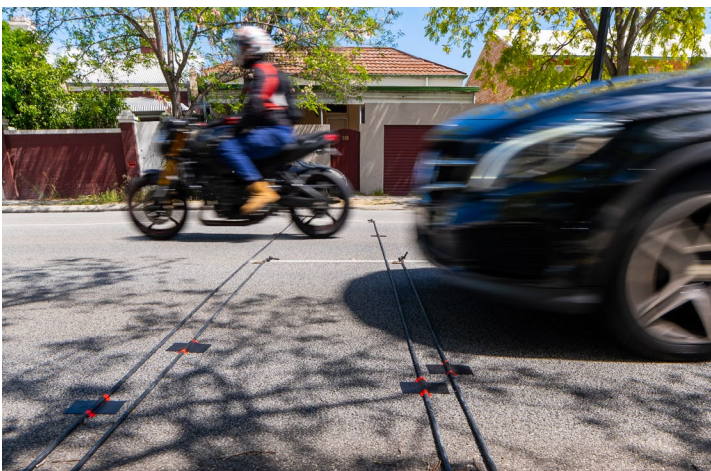
The RoadPod VT4 can classify any type of vehicle according to standard or custom class schemes from around the world.
