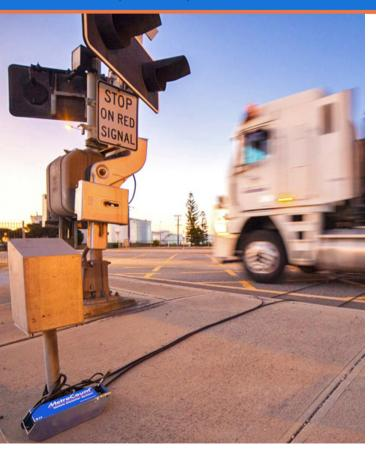
The RoadPod<sup>®</sup> PhaseT simultaneously collects traffic data (via tubes) and signal timings (via fibre optic cable) to paint a clear picture of road activity at traffic signals and rail crossings.
