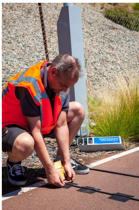
Pic 4. above: Using strips of Bitumen Tape across the length of the tubes to secure the tubes to the Bike path surface
