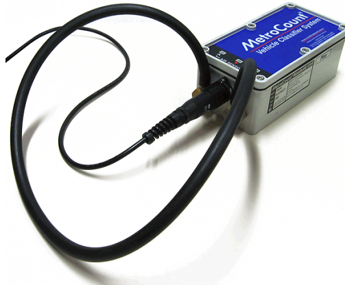
Sensor Hit Test using a short length of tube
